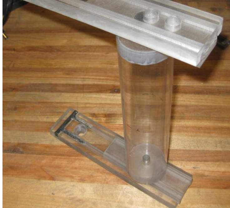
Figure 3-3: Polycarbonate cylinder mounted with sliding mechanism.
