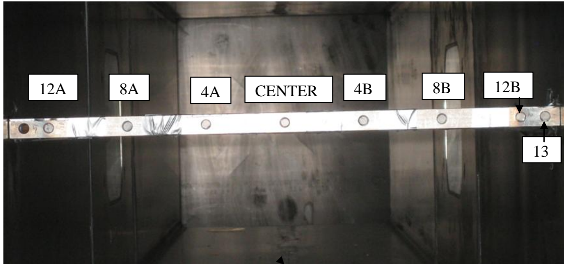
Figure 5-12: Sensor bar used for planarity testing in 28-inch shock tube.
